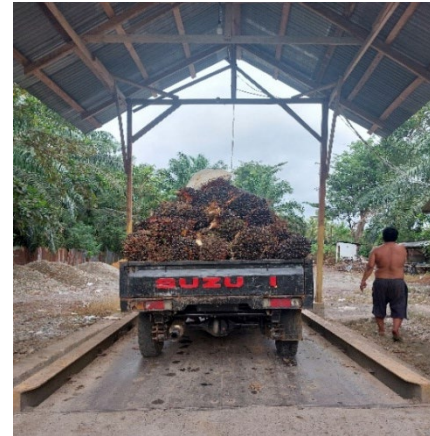
A dealer's truck on a weighing bridge, used to weigh the FFB being brought to a collection yard. Source: Thijs Pasmans
